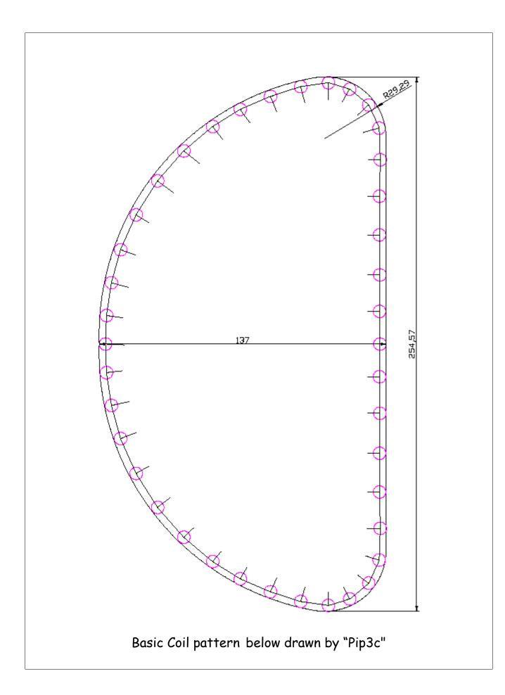
So, how many turns of wire? For this pattern, *I am going to suggest 99 turns for Tx and 104 turns for Rx (30 AWG enameled wire).* In running the calculations for coil inductances a difference of just 5 turns is usually the answer for difference of .5mH between the two coils. I have been able to consistently build "good" coils this way.
