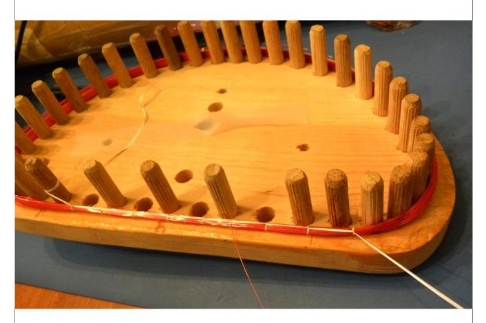
Following constraining the wires, they *must* be infused with cyan glue, so the coils become very stiff. This is very important as IB detectors are very unforgiving if not mechanically rigid!
