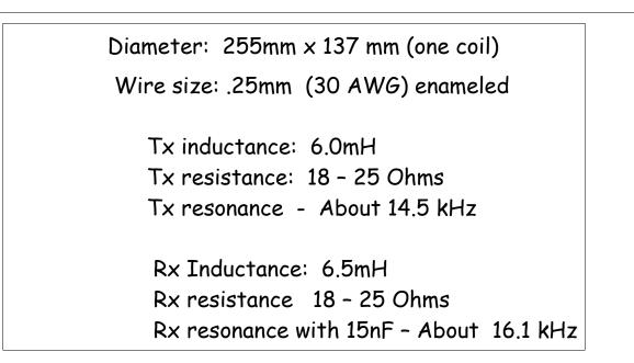
Regardless of the exact dimensions or number of turns, most importantly we *must* have the proper inductances and nulling or phasing will be off and proper ground balance setting and/or disc setting may not be possible.
