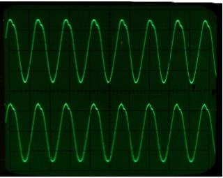
Test point 9 DISC set at Minimum
