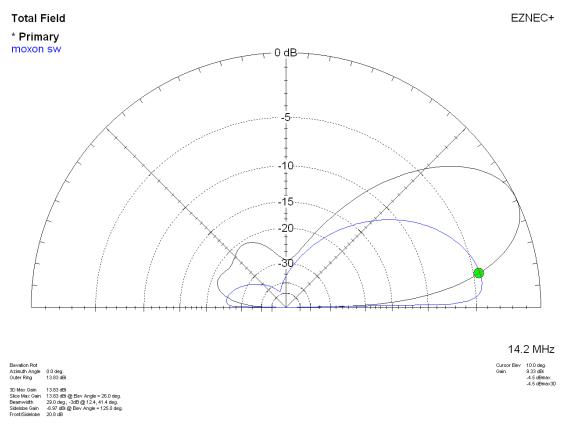
Figure 2 - Comparison of Moxon / Yagi Over Salt Water
