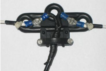
Figure 7 - Dipole Centre Piece
