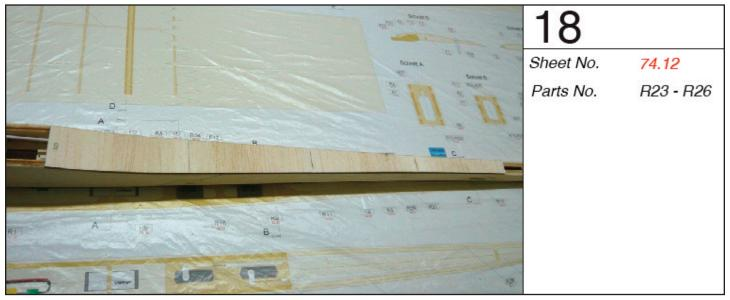
• Glue the rear fuselage cover R23 to R26 starting from the frame R11 & Caution: Be careful to not twist the boom while glueing.
