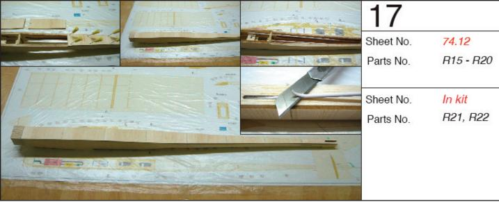
• Glue the bottom of the fuselage R15 to R20 starting from the end of the fuselage and secure with needles.
